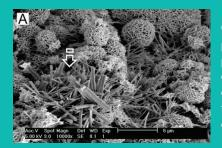
Calcium phosphate precipitated crystals scattered on the hydrated tricalcium silicate cement surface<sup>3</sup>.
