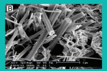
High magnification image of the calcium phosphate crvstals<sup>3</sup>.
